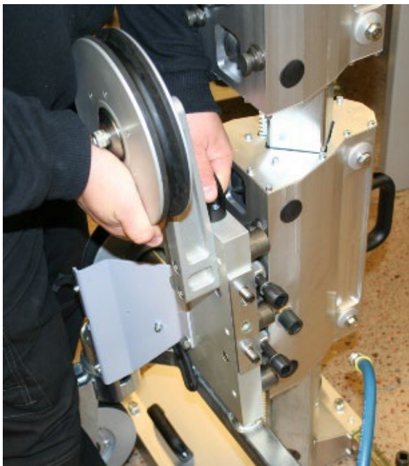
Fitting the lower assembly
